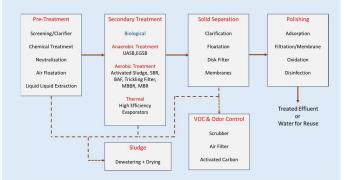
An integrated waste treatment system usually consists of three phases: primary treatment, secondary treatment, and advanced treatment.
