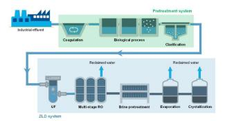
Above shown is the brief representation of UF, RO & ZLD schematic of post treatment of secondary treated water.
